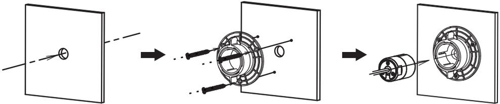
(1) Open a hole with a 3mm in the wall (for cylindrical plate lens, open a 26mm hole in the wall).
