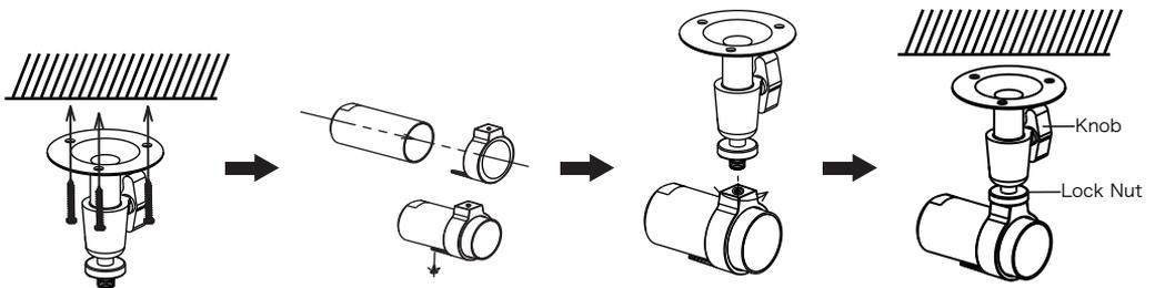
(1) Fix the lens mount 2 to the wall with screws.
